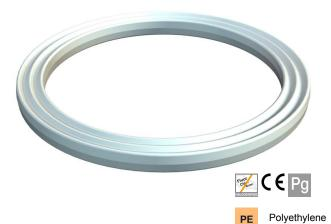
Connection thread sealing ring, in accordance with Part 9 to DIN 46320, however, dimensions may, according to material or function, deviate, suitable for all plastic cable glands with PG connection thread to DIN EN 40430, the internal diameter of the sealing rings are designed so that they can be captively premounted.
