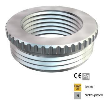
Reduction (Part H) to DIN 46320, with Pg thread to DIN 40430, as a transition from a PG thread hole to a smaller cable gland. \* Prices according to DEL notation.
