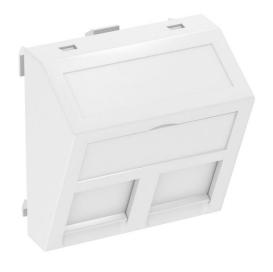
Data technology support with slanting outlet and locking slider to accept two data technology connection modules with RJ45 socket. The locking fastening is suitable for horizontal and vertical installation in the system environment. Type F has a special module seat and is designed for indirect fastening of the data connecti-
