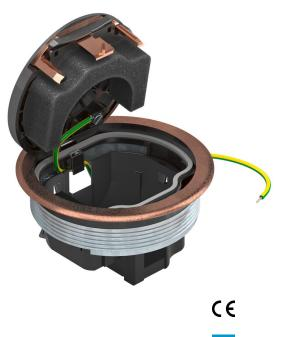
Round installation unit with floor covering protection frame for direct installation in the connection socket UDL2-120 for indoor use. When closed, the installation unit can be wet-cleaned. The minimum installation depth is 70 mm.
