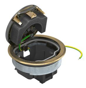
Round installation unit with floor covering protection frame for direct installation in the connection socket UDL2-120. When closed, the installation unit can be wetcleaned. The minimum installation depth is 70 mm.
