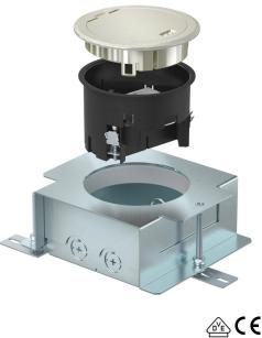
Round GES R2 service outlet with hinged cover, floor covering protection frame and UD GES R2 screed socket for installation in floors with screed structures in internal areas. Installation unit with a double power socket with a 33° insertion direction. At the side, next to the socket, there is space for an optional two connection sockets for data technology applications. When closed, the installation unit can be wet-cleaned. The minimum installation depth is 85 mm. Surface: Nickelplated.
