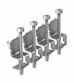
Four universal fastenings for round service outlets and junction box inserts of nominal size R4, R7 and R9 in trunking systems, raised and cavity floors and for rectangular service outlets and junction box inserts of nominal sizes 4, 6 and 9 in trunking systems. Eight universal fastenings are required to fasten the GRAF9 service outlet. Spare part.
