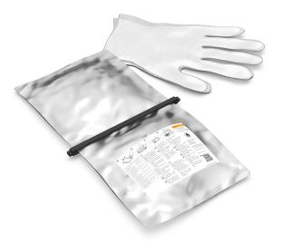
Two-component casting compound Aquasit in an aluminium bag, for filling junction boxes in outdoor areas exposed to high levels of and long-lasting dampness. Also applicable for use against mechanical shock.
