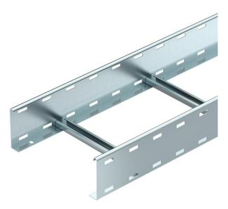
Cable ladder with perforated side rail of side height 110 mm with riveted C profile rungs, open in an upwards direction.
