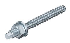
Bolt tie for direct mounting without additional anchors in cracked and uncracked concrete and masonry. With connection thread and washer to accept large loads. Suitable for fastening suspended loads from suspended supports and wall brackets in push-through mounting.
