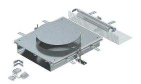
Ready-to-mount trunking extension unit with a device installation lid for the installation of a flush-mount unit of nominal size R9, consisting of the trunking base (floor trough with side and floor covering contact profiles), trunking lid with blank mounting opening and a flushfloor end cover. The scope of delivery contains 3 height-adjustable fixing brackets, 3 screed anchors, 1 lid butt support and 1 construction set for 90° angle
