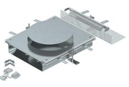
Ready-to-mount trunking extension unit with a device installation lid for the installation of a flush-mount unit of nominal size R9, consisting of the trunking base (floor trough with side and floor covering contact profiles), trunking lid with blank mounting opening and a flushfloor end cover. The scope of delivery contains 3 height-adjustable fixing brackets, 3 screed anchors, 1 lid butt support and 1 construction set for 90° angle.
