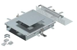
Ready-to-mount trunking extension unit with a device installation lid for the installation of a flush-mount unit of nominal size 9, consisting of the trunking base (floor trough with side and floor covering contact profiles), trunking lid with blank mounting opening and a flushfloor end cover. The scope of delivery contains 3 height-adjustable fixing brackets, 3 screed anchors, 1 lid butt support and 1 construction set for 90° angle.
