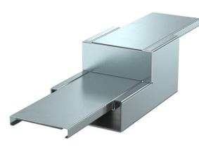
Reducer with intumescent fire protection mesh for symmetrical reduction of straight duct sections from PLM D 0810 to PLM D 0410. Suitable for direct wall and ceiling mounting, mounting below system floors and on support systems. Tool-free joint mounting with PLM SI joint connector. The cover is snapped on without tools, allowing rapid inspection and retroassignment. The cover overhang allows offset cover mounting for continuous equipotential bonding of the entire duct section.
