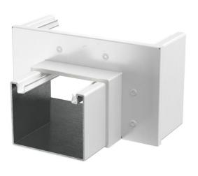
Reducer with intumescent fire protection mesh for symmetrical reduction of straight duct sections from PLM D 1220 to PLM D 0810. Suitable for direct wall and ceiling mounting, mounting below system floors and on support systems. Tool-free joint mounting with PLM SI joint connector. The cover is snapped on without tools, allowing rapid inspection and retroassignment. The cover overhang allows offset cover mounting for continuous equipotential bonding of the entire duct section.
