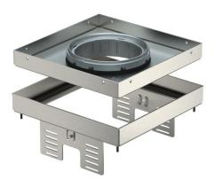
Height-adjustable cassette, decoupled from the floor, of nominal size 4, for tube bodies, for the installation of accessories in dry or wet-cleaned floors for indoor use, for mounting in underfloor boxes UZD250-3 or UZD350-3, either in conjunction with a mounting lid DUG../4 or in UGD250-3/4 or UGD350-3/4. Mounting takes place using height adjustment brackets (order separately) in the aluminium frame profile of the underfloor boxes.
