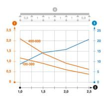
Load diagram, cable tray, type RKSM 60
