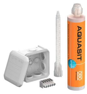
Junction box set with terminal strip for the connection of cables and lines indoors and in outdoor areas exposed to high levels of and long-lasting dampness. Including Aquasit two-component casting compound in a cartridge. Square design with plug-in seals to the sides and knock-out entries in the bottom. Suitable for wall and ceiling mounting and on mounting panels. With the option to fasten inside. With fixed clamping cover. Made from halogen-free materials.
