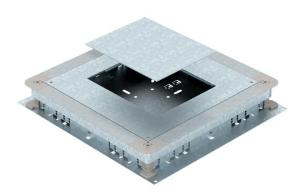
Underfloor accessory box for screed-covered underfloor installation ducts with sheet steel side walls. To mount installation units of the selected nominal size. Height can be infinitely adjusted to the nominal screed height (rapid adjustment possible) and the screed can be worked flush to the screed scraping edge. With noise decoupling option after screed laying and can be used with system accessories, also for heavy-duty application.
