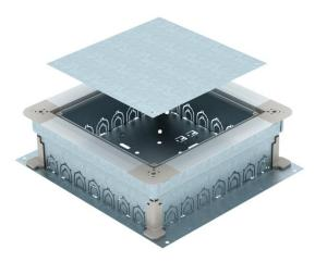
Underfloor junction and branch box for 7 installation pipes on each side (M20 or M32) with sheet steel side walls. To mount installation units in the mounting lid (to be ordered separately). Height can be infinitely adjusted to the nominal screed height (rapid adjustment possible) and the screed can be worked flushed to the screed scraping edge. With noise decoupling option after screed laying and can be used with system accessories, also for heavy-duty application.
