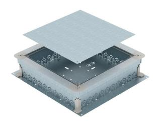
Underfloor junction and branch box for 10 installation pipes on each side (M20 or M32) with sheet steel side walls. To mount installation units in the mounting lid (to be ordered separately). Height can be infinitely adjusted to the nominal screed height (rapid adjustment possible) and the screed can be worked flushed to the screed scraping edge. With noise decoupling option after screed laying and can be used with system accessories, also for heavy-duty application.
