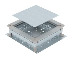
Underfloor junction and branch box for 7 installation pipes on each side (M20 or M32) with sheet steel side walls. To mount installation units in the mounting lid (to be ordered separately). Height can be infinitely adjusted to the nominal screed height (rapid adjustment possible) and the screed can be worked flush to the screed scraping edge. With noise decoupling option after screed laying and can be used with system accessories, also for heavy-duty application.
