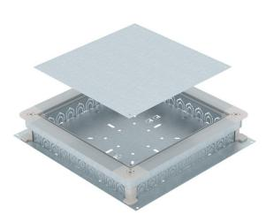
Underfloor junction and branch box for 10 installation pipes on each side (M20 or M32) with sheet steel side walls. To mount installation units in the mounting lid (to be ordered separately). Height can be infinitely adjusted to the nominal screed height (rapid adjustment possible) and the screed can be worked flush to the screed scraping edge. With noise decoupling option after screed laying and can be used with system accessories, also for heavy-duty application.
