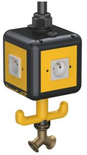
Housing equipped and pre-wired, with 1 m pipe 1/2" and connection for compressed air hose 13 x 3.5 mm and 2-way distributor 1/2", with suspension lug, grip hook and four cover plates.
